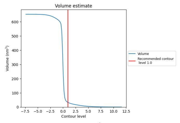
The volume at the recommended contour level is  $32 \text{ nm}^3$ ; this corresponds to an approximate mass of 29 kDa.
