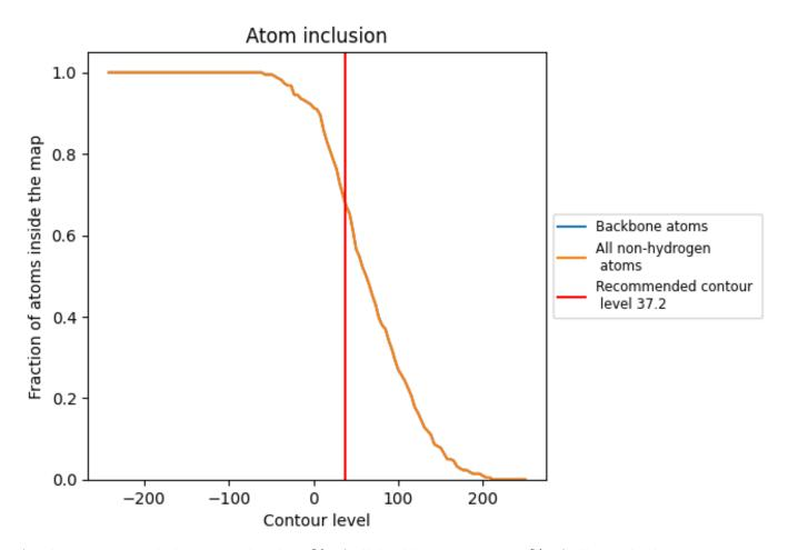
At the recommended contour level, 68% of all backbone atoms, 68% of all non-hydrogen atoms, are inside the map.
