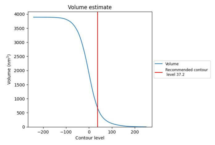
The volume at the recommended contour level is  $681 \text{ nm}^3$ ; this corresponds to an approximate mass of 615 kDa.
