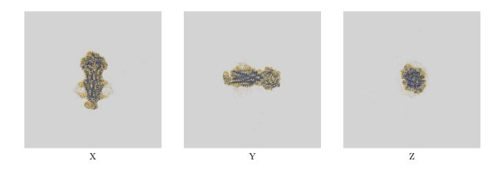
The images above show the 3D surface view of the map at the recommended contour level 0.32 at 50% transparency in yellow overlaid with a ribbon representation of the model coloured in blue. These images allow for the visual assessment of the quality of fit between the atomic model and the map.
