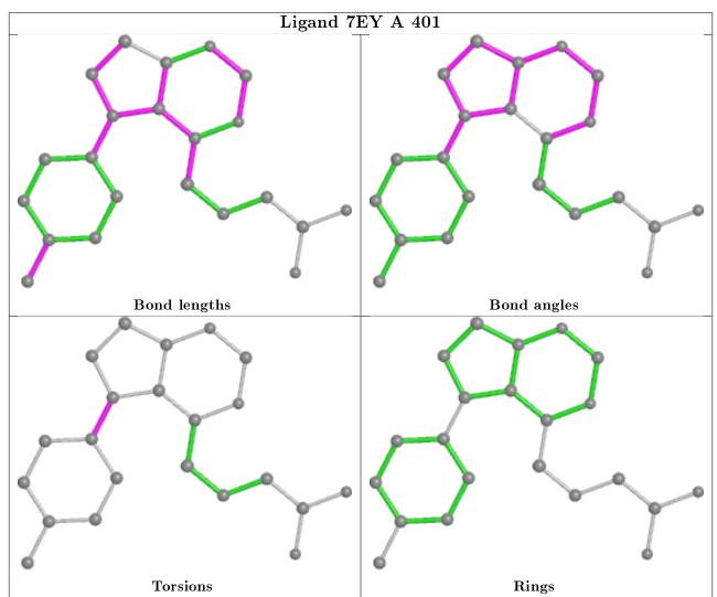
The outliers are highlighted in purple. The color gray indicates Mogul did not find sufficient equivalents in the CSD to analyse the geometry.
