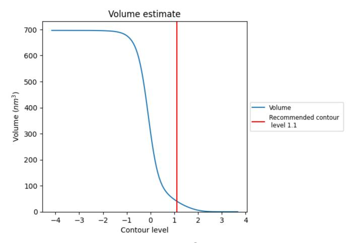
The volume at the recommended contour level is 41 nm<sup>3</sup>; this corresponds to an approximate mass of 37 kDa.
