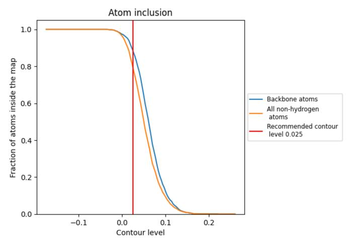
At the recommended contour level, 89% of all backbone atoms, 80% of all non-hydrogen atoms, are inside the map.
