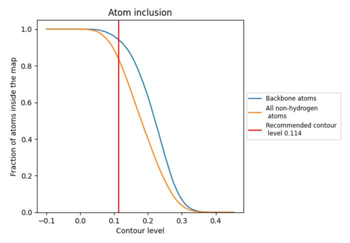
At the recommended contour level, 94% of all backbone atoms, 83% of all non-hydrogen atoms, are inside the map.
