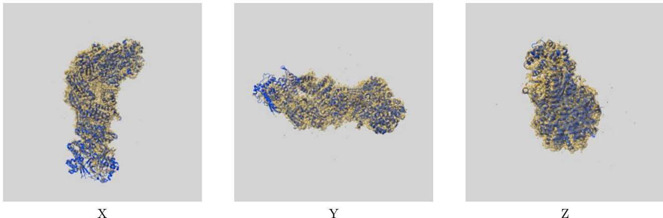
The images above show the 3D surface view of the map at the recommended contour level 0.067 at 50% transparency in yellow overlaid with a ribbon representation of the model coloured in blue. These images allow for the visual assessment of the quality of fit between the atomic model and the map.
