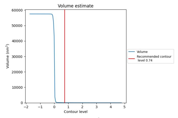
The volume at the recommended contour level is  $54 \text{ nm}^3$ ; this corresponds to an approximate mass of 49 kDa.
