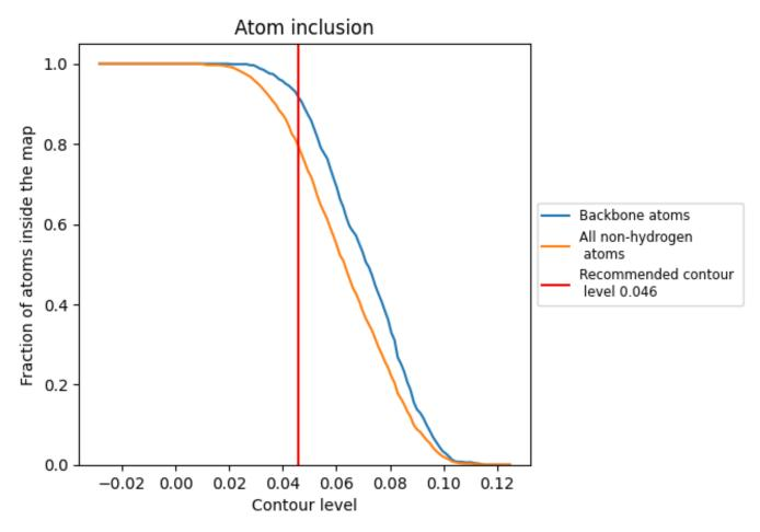
At the recommended contour level, 92% of all backbone atoms, 79% of all non-hydrogen atoms, are inside the map.
