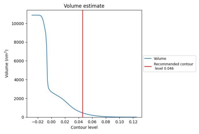
The volume at the recommended contour level is 446  $\text{nm}^3$ ; this corresponds to an approximate mass of 403 kDa.
