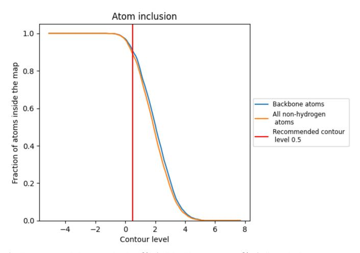
At the recommended contour level, 91% of all backbone atoms, 89% of all non-hydrogen atoms, are inside the map.
